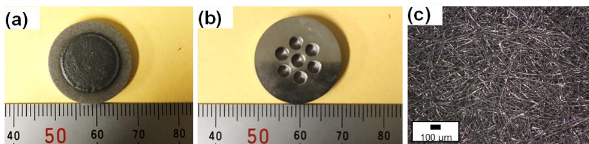
Fig. 3 Images of metal supported mesh cell, MM500Y#1, (a)anode side, (b)cathode side, (c)part of mesh
